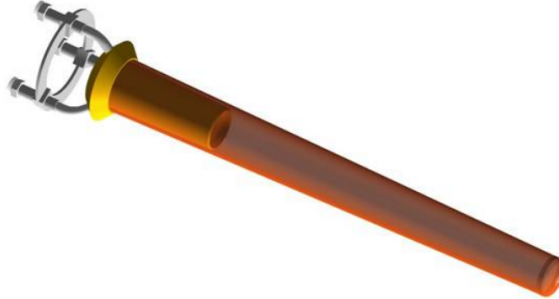
Figure 2.5: Diagram of the g12 cryotarget, filled with liquid Hydrogen. Image source: [14].
