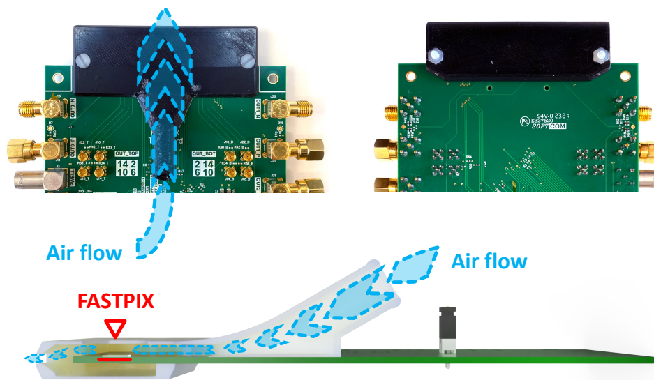
Figure 6.4: ABS plastic 3D printed chip cover. The top left and top right show the installed cover from the front face and backside of the PCB. The bottom image illustrates the air flow inside of the cover rendered in a light grey material.
