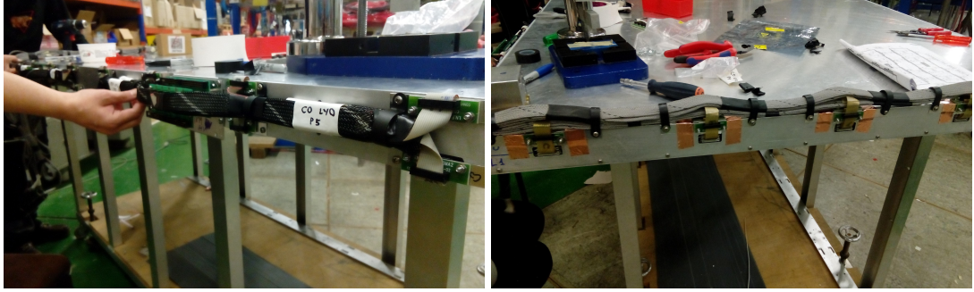
Figure I.2 Cabling of the BME chambers.
