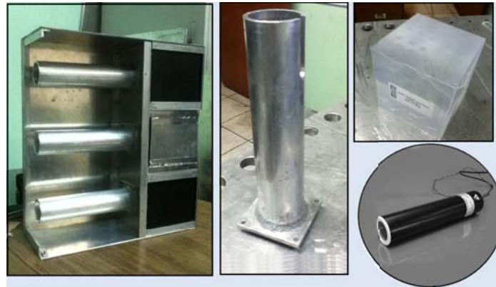
Figure 1. Left to right: Three channel detector internal structure, aluminum tube where the photomultiplier is introduced, plastic Scintillator Saint-Gobain BC-408 [3] and Sens Tech photomultiplier P30CW5[4].
