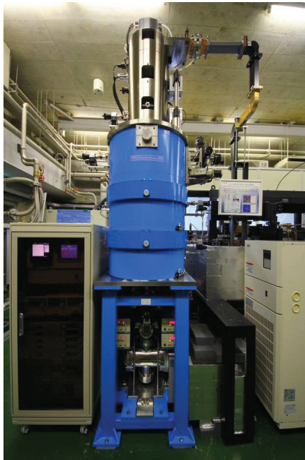
Figure 1: Prototype of femtosecond time-resolved relativistic-energy electron microscopy using RF gun.
