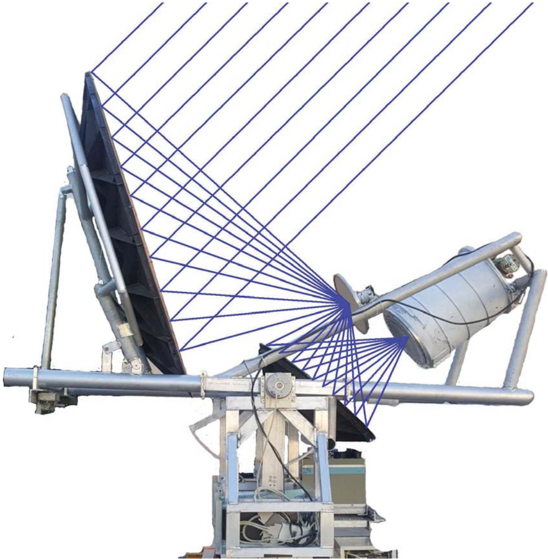
Figure 4.4: Sketch of optical path with baffles removed.
