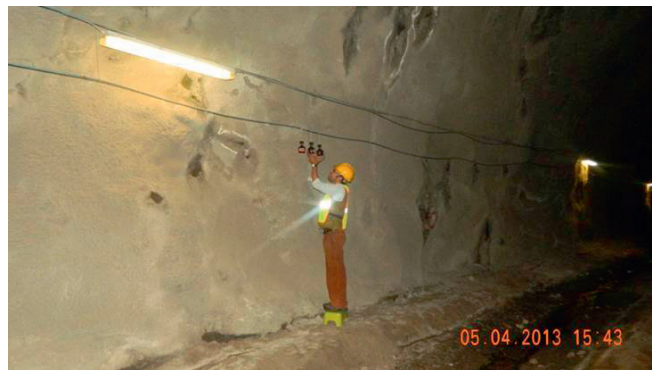
Figure 2. Electrets mounted in groups of 3 on the walls of the tunnel close to the vehicle cross-cuts.
