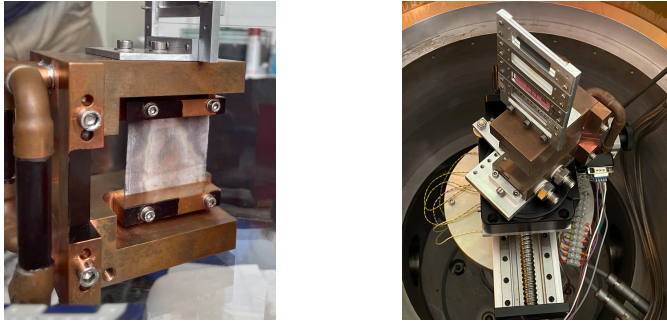
Figure 3. High-luminosity lithium target used for the hypertriton experiment. Left: The lithium sheet has a thickness of 2.5 \text{ g/cm}^2 in beam direction. In the left part of the setup, pipes for the cooling liquid can be seen for the optimal removal of heat from the lithium sheet. Parts of the copper frame are painted with infrared absorbing black paint to prevent undesired reflections in the camera pictures. Right: The copper frame mounted inside the target chamber, additional targets on top. Below the frame, a rotary and a linear stepper motor are located.
