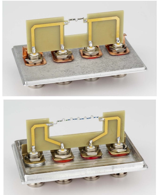
Figure 6. Photographs of the opened case with four series-connected SMD resistors named 4S1 (top) and twelve series-connected SMD resistors named 12V1 (bottom). The centre distance of two adjacent BNC connectors is 22 mm and can be used as a scale.
